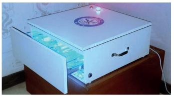
The Research Centre Imarat (RCI), a laboratory of DRDO based in the city, has developed an automated contactless UVC sanitisation cabinet Defence Research Ultraviolet Sanitizer (DRUVS).
